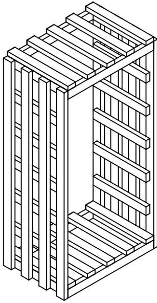
2. Nail only the bottom shelf to the side rail. Leave the top shelf to keep the spacing.
