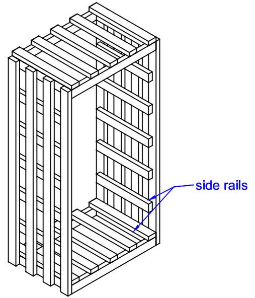
3. Keep adding shelves from the bottom up and nailing them on. Securing the top last.
