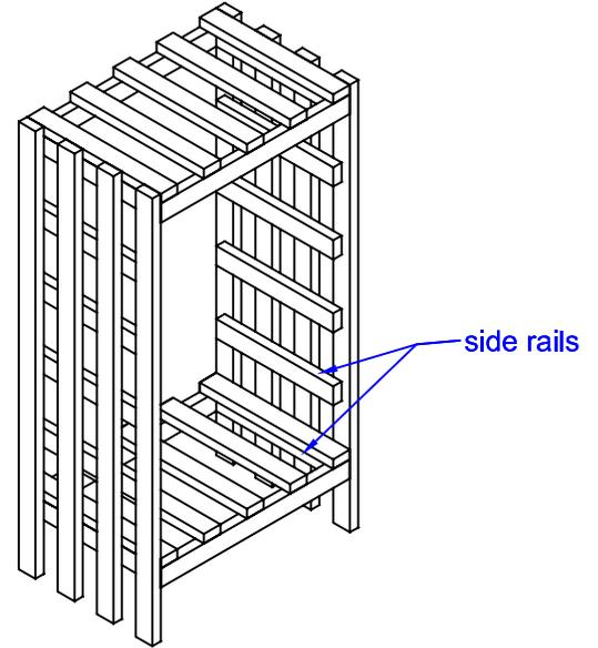
3. Keep adding shelves from the bottom up and nailing them on. Securing the top last.
